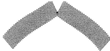
Fig. 12 Deformed state of thin specimen with notch at \theta=45^\circ
